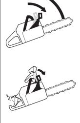
7 During felling your left hand grasps the front handle in such a way that it cannot activate the front hand guard. In this position the chain brake can only be activated by the inertia action of the counterweight.
